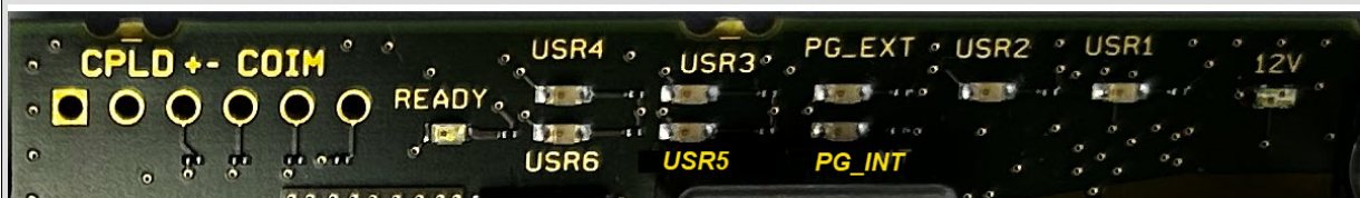
Figure 27.26. LEDs on the imaFlex CXP-12 Penta Board
