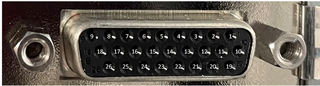
Figure 27.21. Front GPIO Connector of the imaFlex 2 Dual 100
