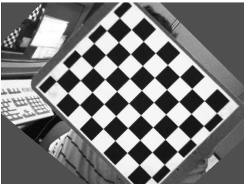
Figure 10.87. Rotated, distortion and Keystone corrected target image
